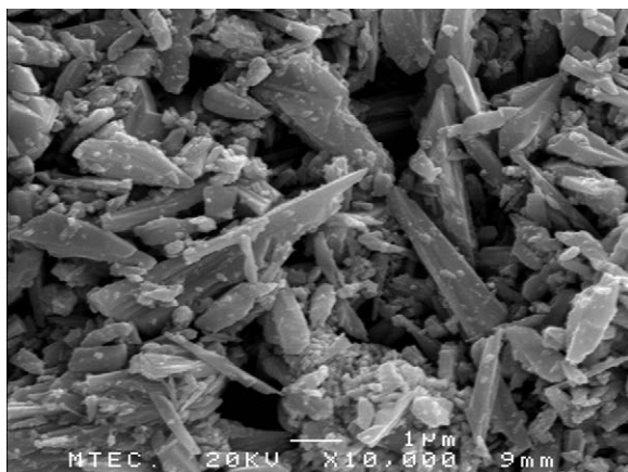
Fig. 4. SEM image of SnO 2 prepared from 0.188 [Na 2 SnO 3 ·3H 2 O]/0.5 M [NaOH].
